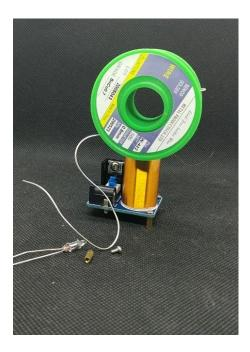
**8.** Now solder the inserted wire to the PCB. You can remove the enamel from the wire by setting the soldering iron to 400 F and with a clean tip running it across the wire. This will burn off the enamel and expose the wire to be soldered.
